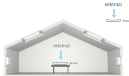
Figure 1.21. Drawing showing the values measured in the daylight factor method (simultaneous reading of the internal and external (unobstructed) illuminance levels on a horizontal plane).
